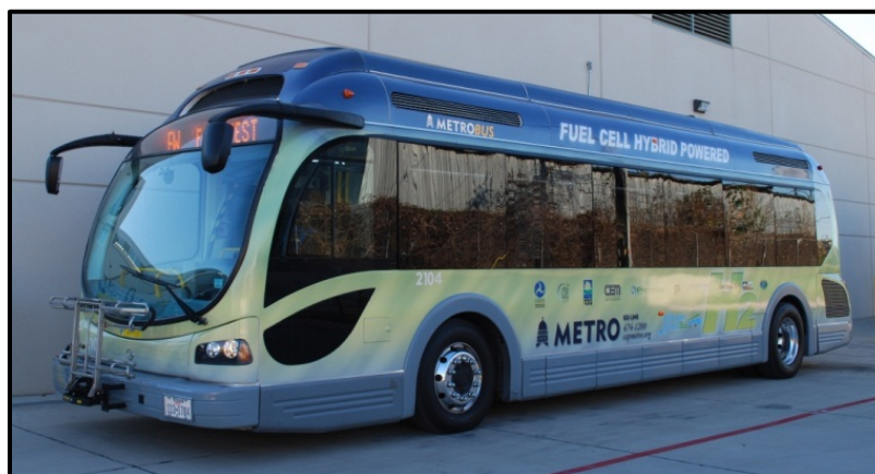
Figure 4. Battery dominant FCEB included in the data summary: Proterra bus in Austin, Texas
