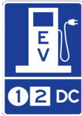
Figure 6. Adaption of EV signage to reflect availability of specific alternating current (AC) charge levels (1 and/or 2) or direct current (DC) fast charging
