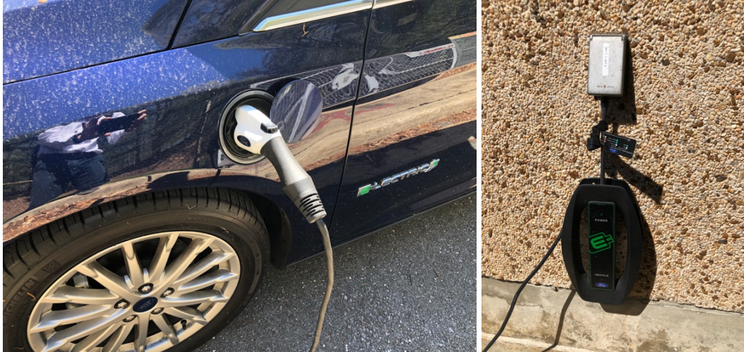
Figure 4. EV at Adelphi Laboratory Center connected to 120-V outlet
