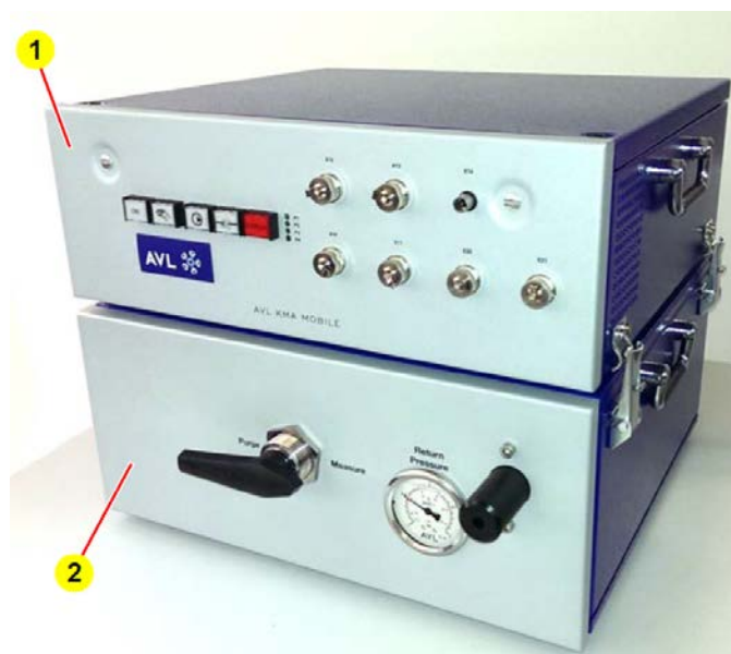
Figure 1. AVL KMA Mobile, 1 – Measuring Module, 2 – Conditioning Module
