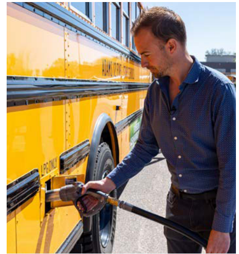
Fueling a propane vehicle is similar to fueling a conventional vehicle and takes about the same amount of time. Some attendant training is required, however. Photo by Werner Slocum, NREL 57379.
